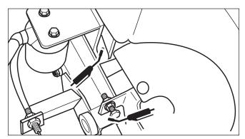
Figure 23. Suspension & Deck Lift Pivots
